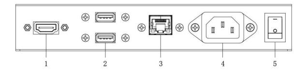
1. HDMI input; 2.USB interface; 3.RJ45 interface; 4.Power port; 5.Rocker switch button;
