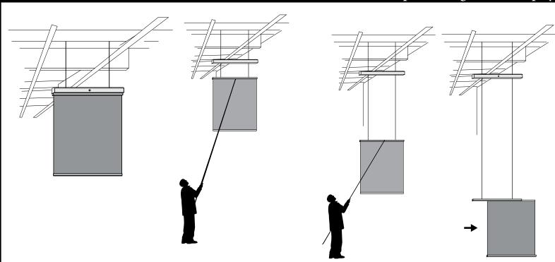
Attach banner hanger to many different types of open ceilings. No ladder is necessary to change your signs. Simply use a pole to lower banner to comfortable height, change banner and then use pole to fully retract. Banner stays in place with powerful magnets.
